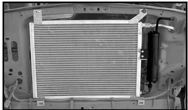
Photo B2 - Mount Condenser Assembly
