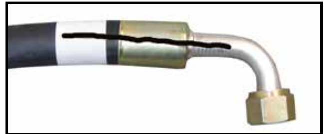
Photo 6 - Mark Position of Fittings on Hose
