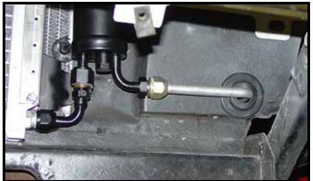
Photo A3 - Drier Inlet Tube
