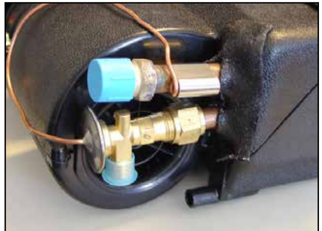
Photo 1 - Install Expansion Valve
