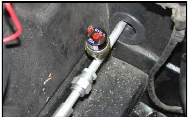
Photo A4 - Pressure Safety Switch
