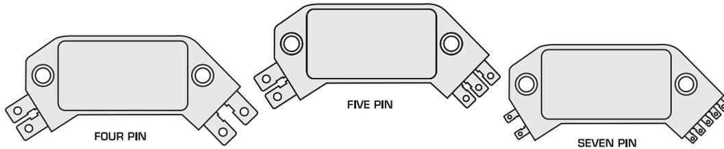
There are three different large cap HEI distributors. To identify which of the following diagrams fit your specific application, remove the distributor cap and rotor and locate the ignition module at the base of the distributor. Count the number of terminals on both ends of the module and follow the corresponding diagram. GM used 4, 5 and 7-pin modules in these distributors.
