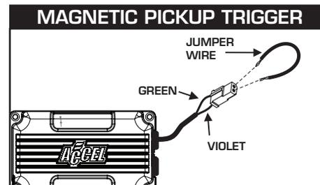
**Figure 8 Checking for Spark with Magnetic Pickup.**
