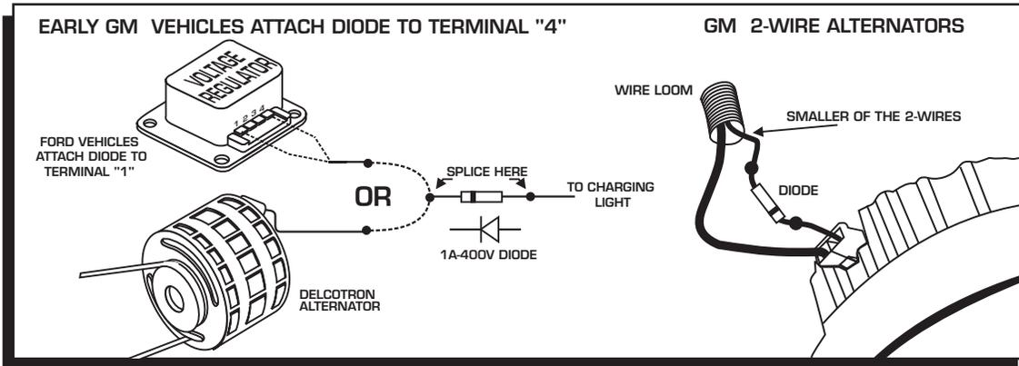
**Figure 5 Installing the Diode to fix Run-On.**
