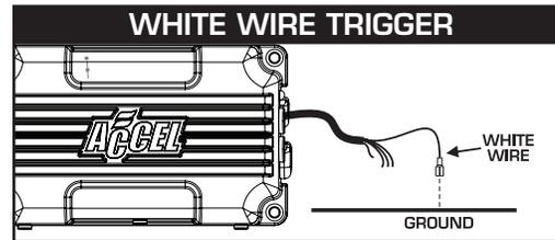
**Figure 7 Checking for Spark with the White Wire.**
