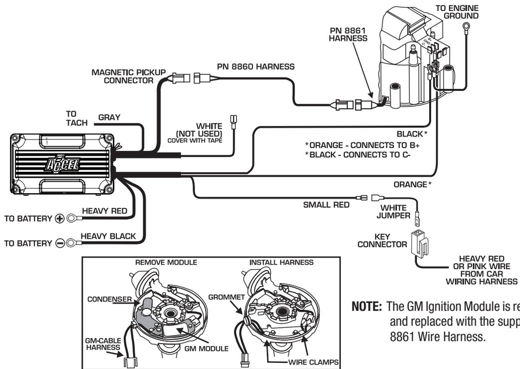
**NOTE:** The GM Ignition Module is removed and replaced with the supplied PN 8861 Wire Harness.
