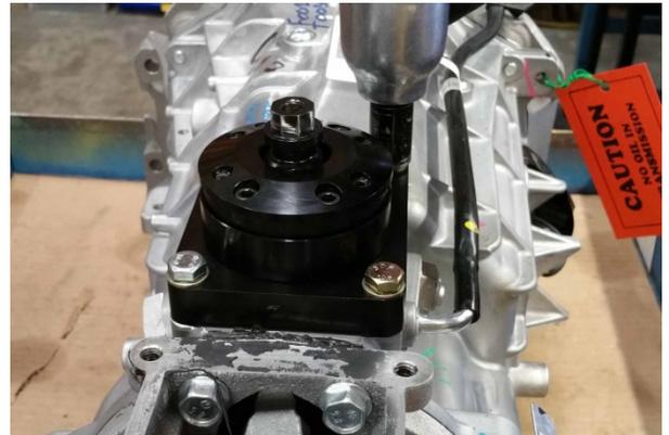
11. Apply a bead of RTV to rear cover flange.
