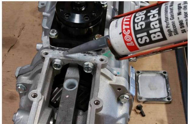
12. Install rear cover and bolt in place using supplied hardware.
