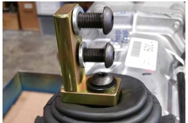
15. Installation is complete and ready to place into the vehicle. This shifter locates the handle in nearly the same location as the stock shifter hole in the floor. There may be some modification required to the floor or tunnel area to accommodate the larger size of the Tremec transmission.
