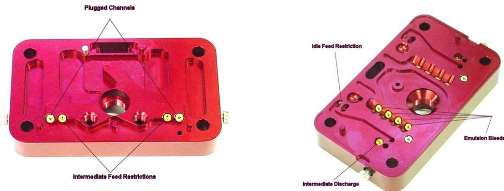
The intermediate system has a feed and discharge restrictions. The feed is located on the fuel bowl side of the metering block (location shown above). The discharge side is on the main body side of the metering block as shown. The idle feed restriction is located at the top of the serpentine channel. The emulsion bleeds are the four restrictions located in the high speed air bleed channel closest to the power valve. The lowest port on the metering block face should be plugged.
