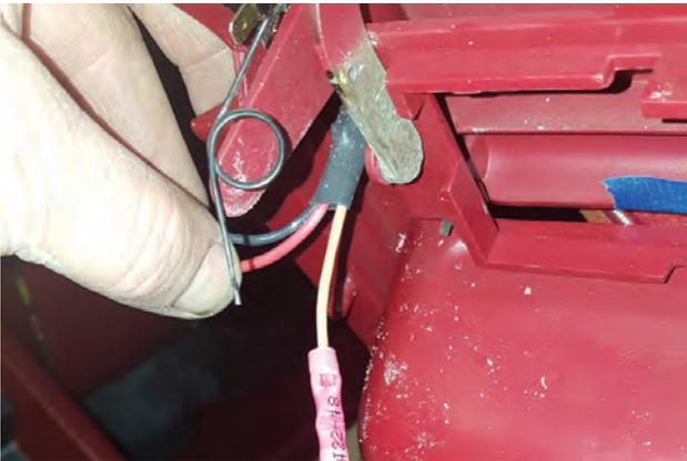
15. Use **splice (13)** to connect solenoid power wire (that was routed through firewall to center console) to brown wire on lit momentary switch.
