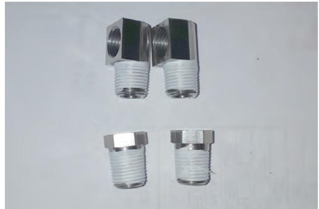
4. Teflon tape on pipe threads must not block fluid flow.
