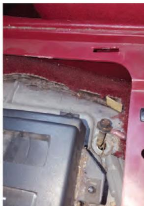
16. Extend momentary switch black ground wire with **splice (13)**, **black wire (5)** and **eyelet (12)**. Ground this wire to chassis (this kit was grounded at shifter).
