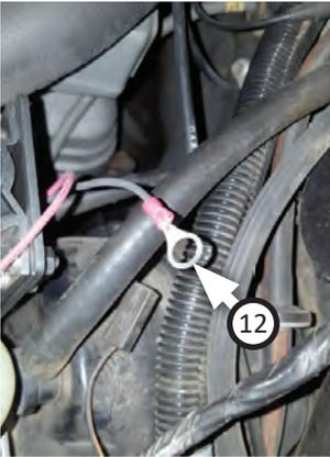
10. Ground solenoid to bracket using eyelet (12).
