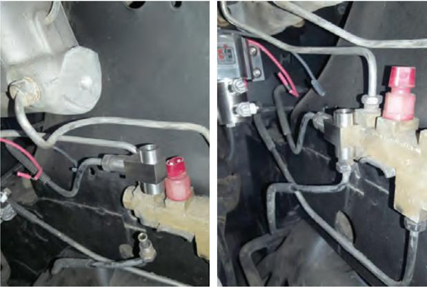
7. Install (x2) front brake lines (removed step 1) into T as shown.
