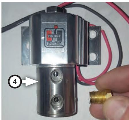
3. The brass plug can be removed and replaced on valve solenoid (4).
