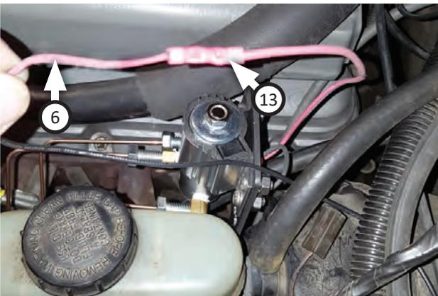
11. Use red wire (6) and splice connector (13) to extend power wire so it will reach from solenoid to vehicle interior.
